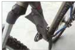
V-9988-DF Tablet Fender, Material PP Assemble in downtube Thickness : 1.0mm PAT.
