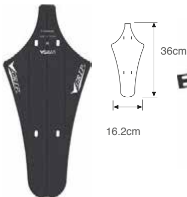
V-9988-XDF Tablet Fender Material PP Assemble in downtube Thickness : 1.0mm
